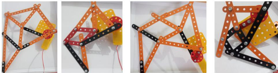
Figure 16: Four Tested Jansen Linkage with Different Dimensions
