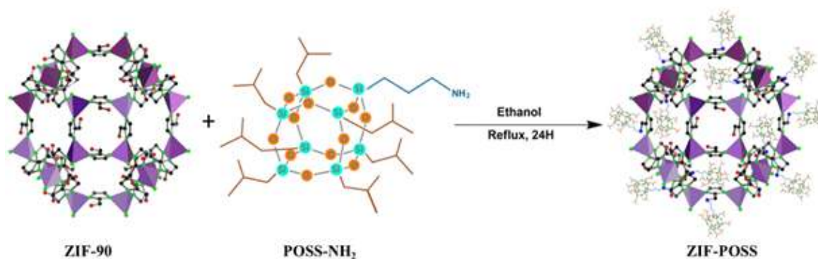
Scheme 6: Synthesis of the ZIF-POSS hybrid material
