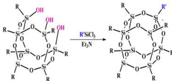
Scheme 3: Corner capping reaction
