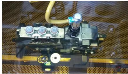
Figure 2: FIP Immersed in oil and connected hoses
