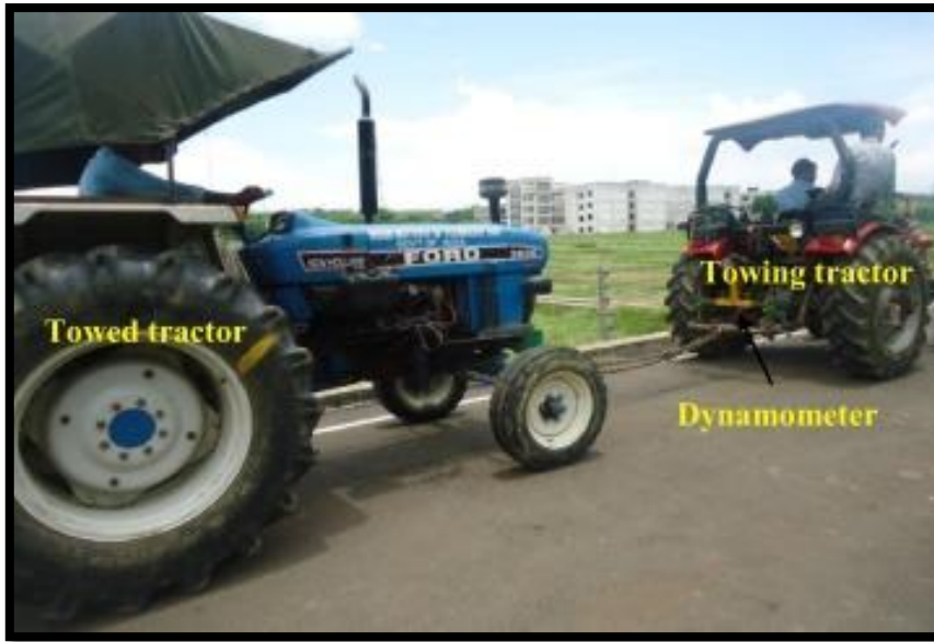
Figure 1: Slip Measurement with Towing and Towed Tractor
