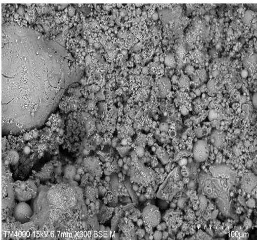
Figure 14: SEM images of sintered pellets.
