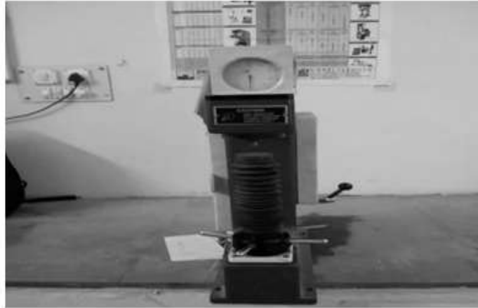
Figure 4: Hardness tester used for Brinell hardness number measurement
