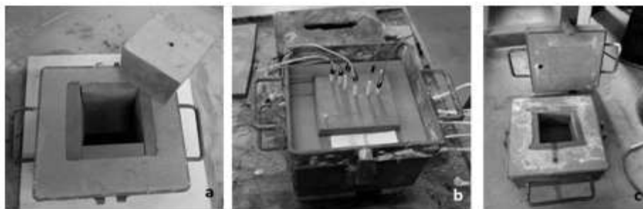
Figure 2: Sand molds (a) With insulating pad and pattern (b) with insulating pad and thermocouples (c) without thermocouple and with insulating pad
