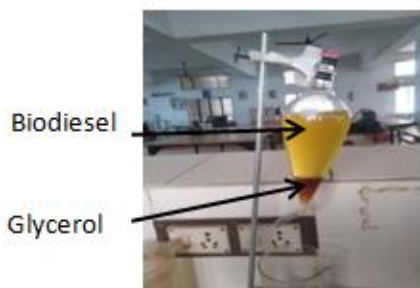
Figure 2: Separation of Glycerol and Esters
