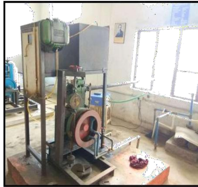
Figure 4: Four Stroke, Single Cylinder, Vertical Diesel Engine
