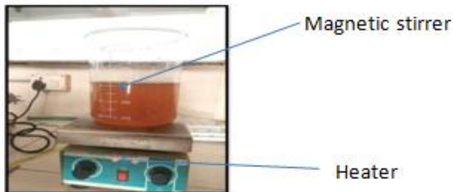
Figure 6: Blending of Oils using Magnetic Stirrer
