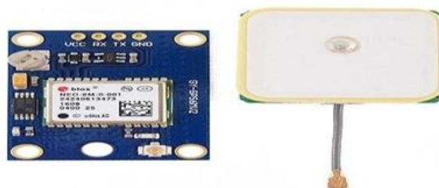
Figure 10: GPS (Ublox Neo 6M)
