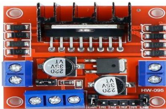
Figure 9: L298N Motor Driver
