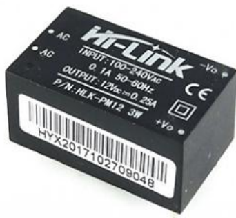
Figure9: Shows Switch Mode Power Supply
