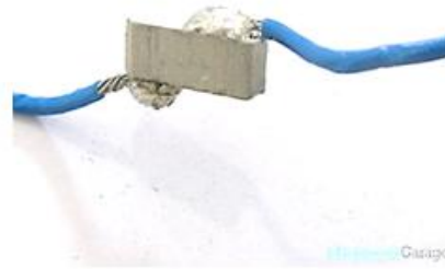
Figure 8: Shows Thermistor with Wires Soldered
