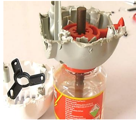
Figure 4: Shows the arrangement of Wick Holds Liquid Bottle
