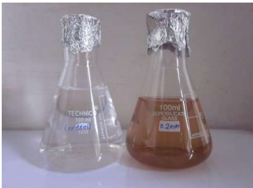
Figure 1: Conical Flasks Containing the Aqueous Extract Before To (Left Flask) And Following The 12-Hour Reaction With \text{Ag}^+ (Right Flask).
