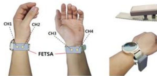
Figure 2: Fabricated sensor array and gesture recognition device based on FETSA.
