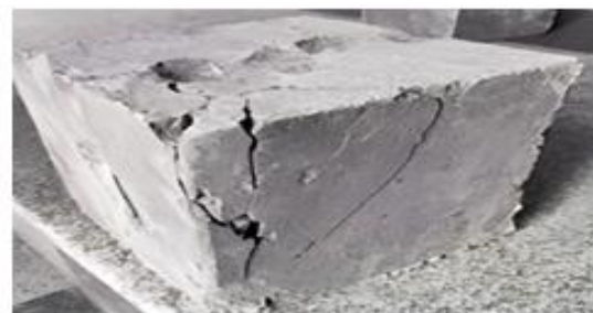
Figure 6: Damaged Concrete Cube
