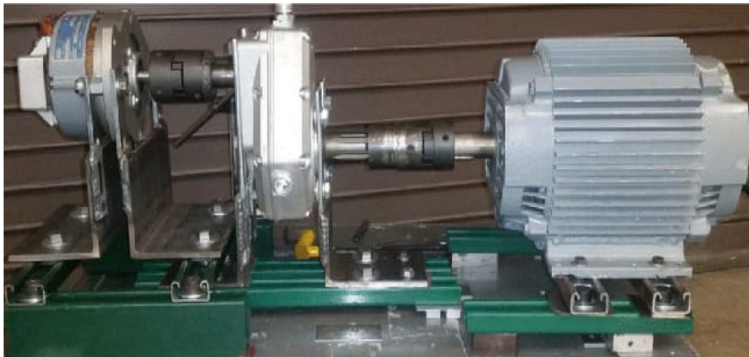
Figure 3: (Alternator with Gear Box- RPM needed-1490-1510)
