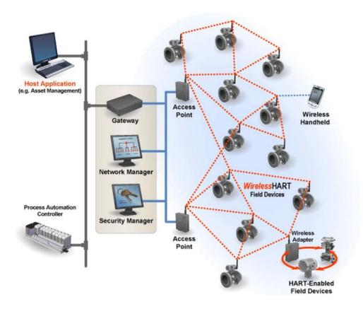
The OSI Model for HART with the physical layer adopts the IEEE 802.15.4-2006 .this also work on the MESH topology
