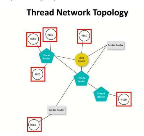
Thread Architecture is consisting of Border Router, Lead Devices, Thread Routers and REED.
