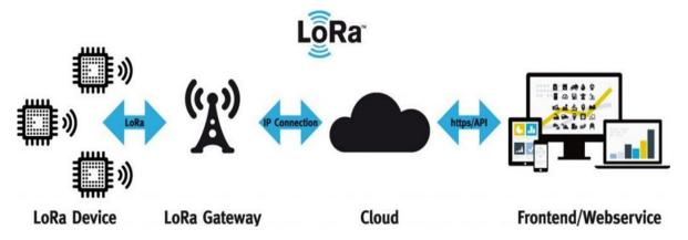
LoRa works on the spread spectrum technology using the unlicensed sub-GHZ band. The LoRa chirp spread spectrums (CSS) modulations ensure full bidirectional communication (get and Post), The LoRa Signals are generated at very low noise levels. It enables high interference resilience but very difficult to detect or jam.
