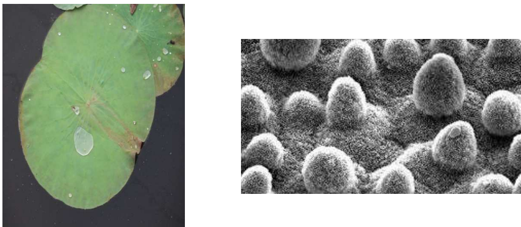
Figure 2: Lotus leaf with SEM Image of leaf surface
