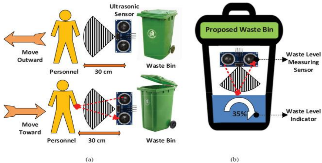
Figure 6: Sensor and Indicators Working Flow Chart
