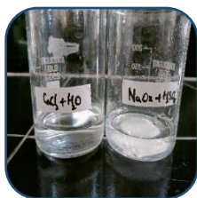
A - Preparation of equimolar solutions of sodium oxalate & \text{CaCl}_2 ,
