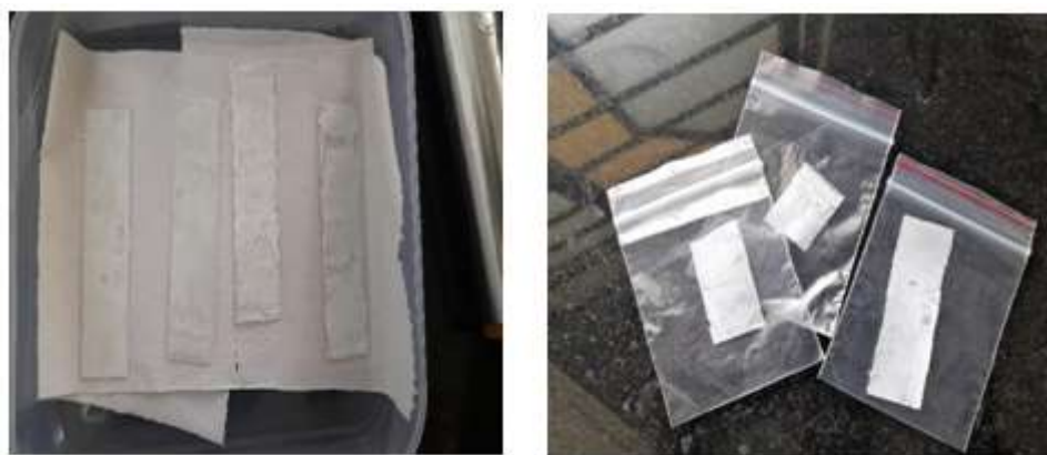
Figure 2: Ps/ TiO 2 Thin Films the image shows the material coated in a substrate and peeled off from a substrate.
