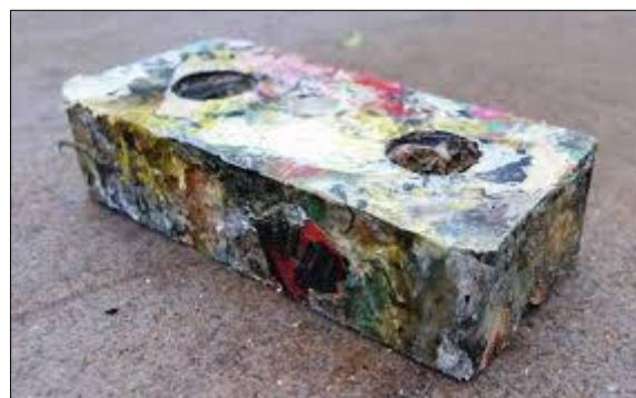
Figure 8: Interlocking brick made with waste plastic
