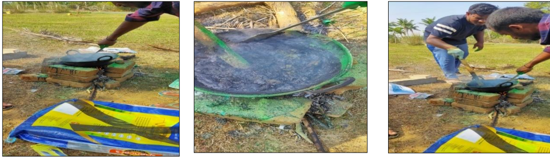
Figure 7: Process of making interlocking plastic brick with a least expensive method
