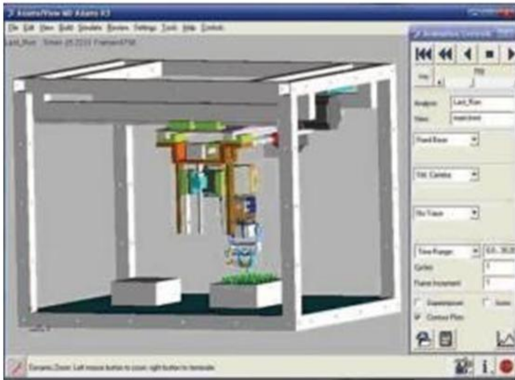
Figure 5: Robotic Teeth Arranger of the Cartesian Kind, Digital Model.
