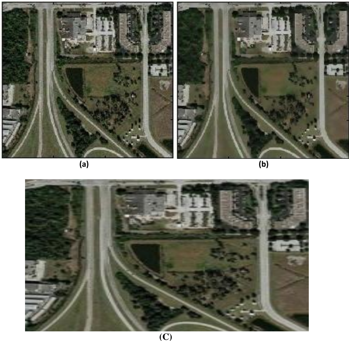
Figure 2: (a) Input Image of Emerging Suburban Area (b) Result of Bilateral Filtering (c) Histogram Equalization Processed Image
