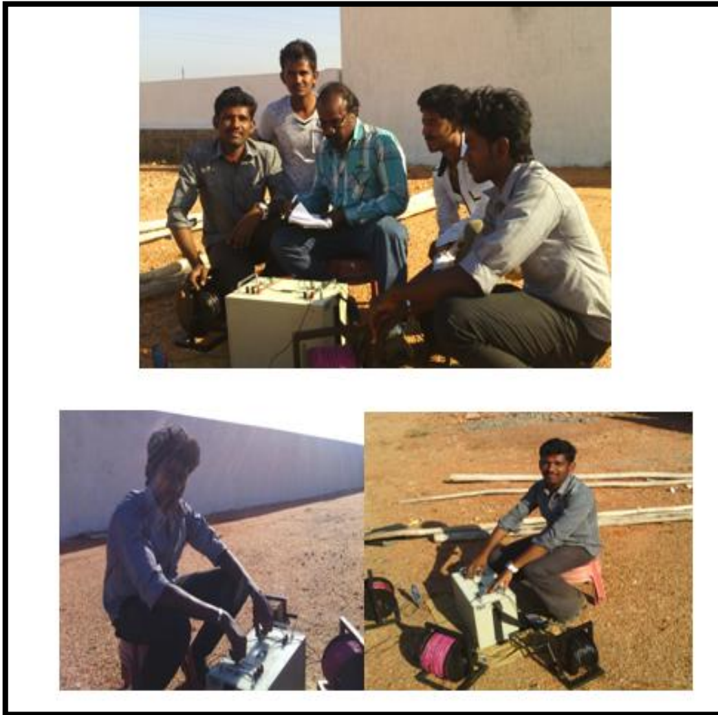
Figure 2: Resistivity Data Collection on the Field.
