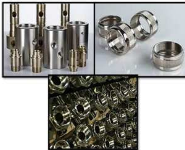
Figure 2: Practical examples of Ni-P Coating of Steel-based Materials
