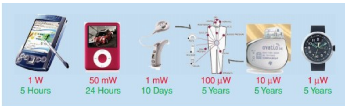
Figure 11: Power Requirement of some Portable Devices [40].
