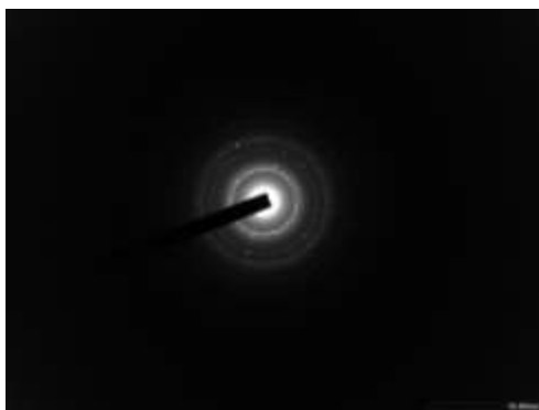
Figure 7: [D] Selected area electron diffraction (SAED) pattern of PVP-b-AgNPs
