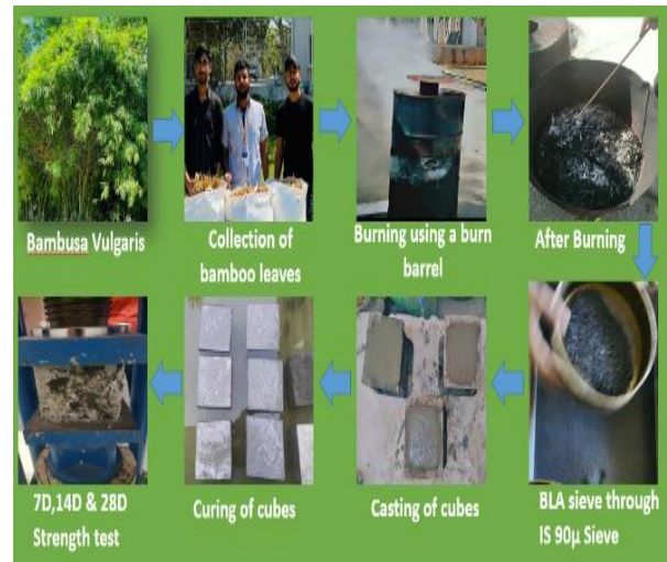
Figure 5: Process of Testing of Cubes Using BLA
