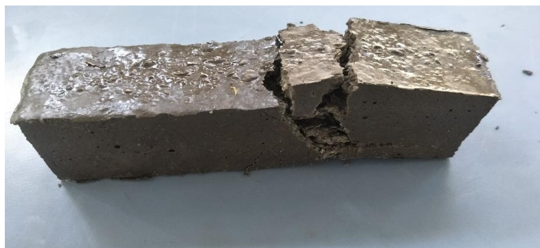
Figure 11: Crushing pattern of 50x50x200mm beam during flexural strength test using 2-hour age sample.
