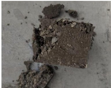
Figure 9: Crushing pattern of 50mm cube during compressive strength test for 2-hour age sample.
