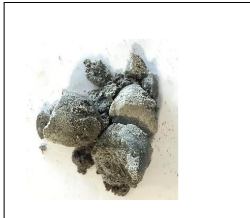
Figure 5: Ratio of diluted resin to silica fume, 1:1.5.
