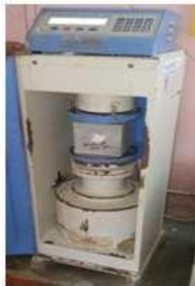
Figure 9: Compressive Strength test of the sample cubes
