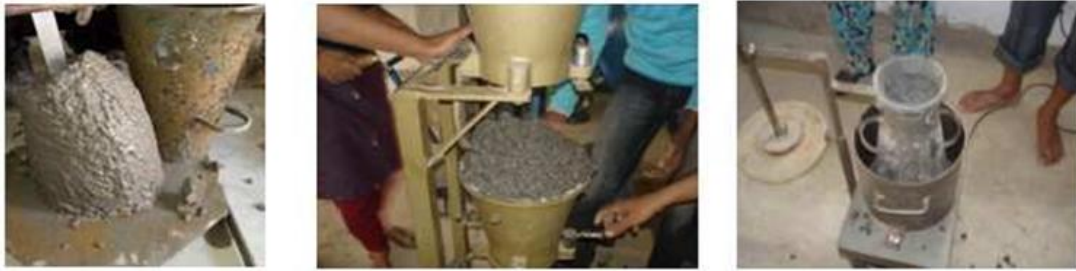
Figure 7: Work ability measurement of all concrete mixes
