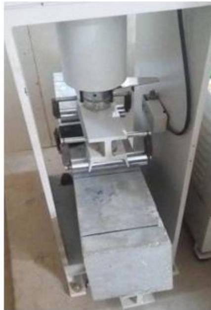
Figure 12: Flexural Strength test of beam specimen
