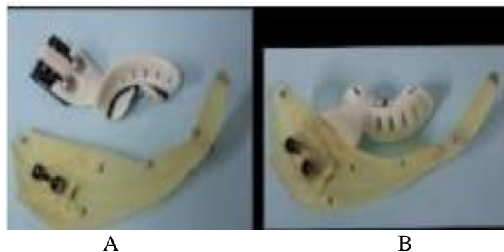
Figure 13: A) Displaying the Yomi patient splint, accentuated with a contrasting insert and fiducial array. B) Yomi fiducial array which is shown connected to patient splint.
