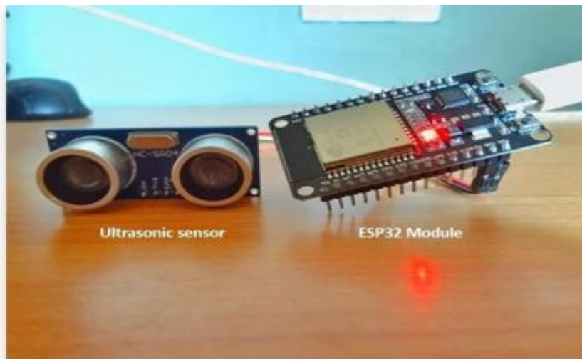
Figure 7: ESP32 connected with ultrasonic sensor.
