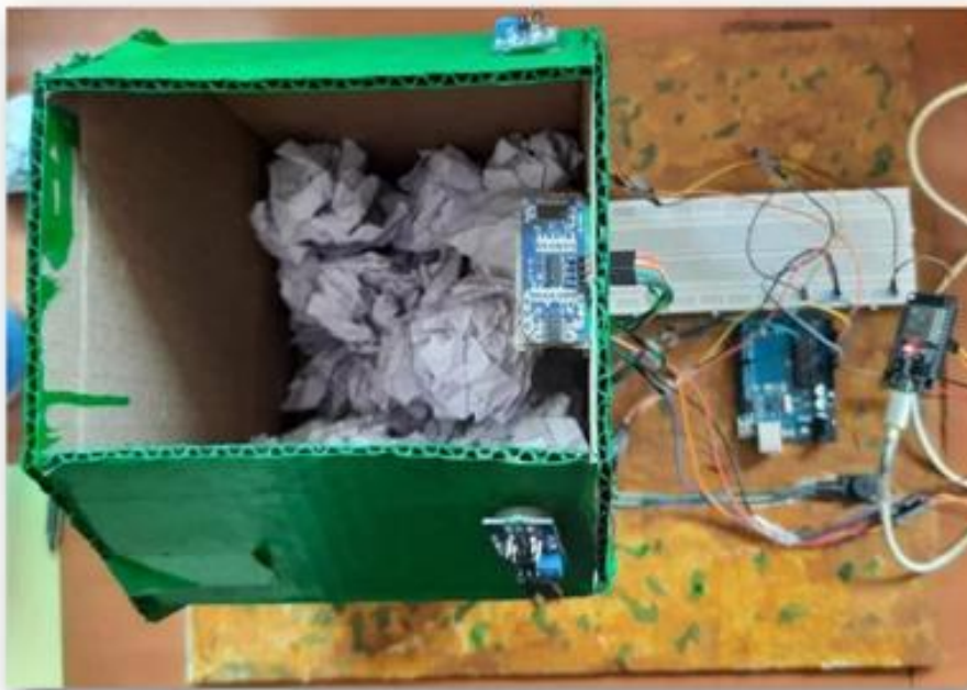
Figure 11: The above snapshot gives the overall top view of the garbage monitoring system
