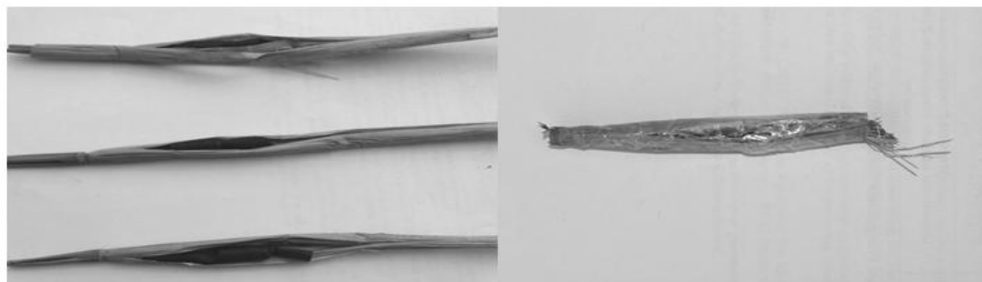
a. Heat sunk rubber-magnet within the inter node of crop b. Taped magnet recovered after threshing
