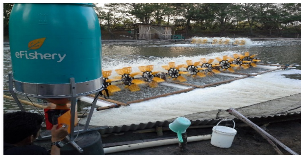
Figure 1: e Fishery AI fish feeder (source :Krishi jagran)
