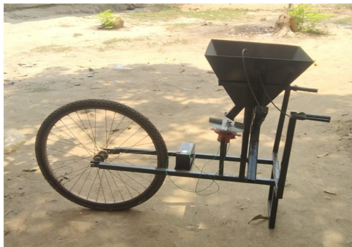
Figure 13: Fabricated Model of Fertilizer Spreader Machine
