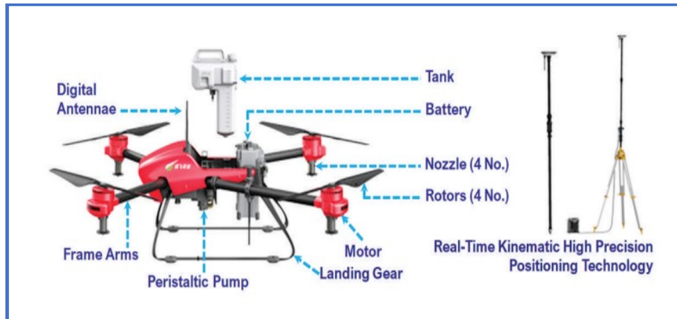
Figure 4: Different Spare Parts of a Drone
