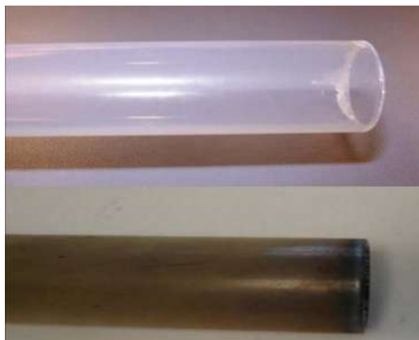
Figure 5: Photograph of TiO 2 and Ag/TiO 2 Photocatalytic Wall Systems
