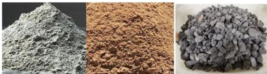
Figure 1: Cement (OPC), Sand, Aggregate
