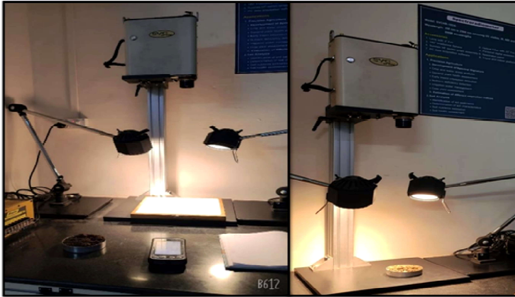
Figure 3: Experimental setup for recording reflectance of soil
