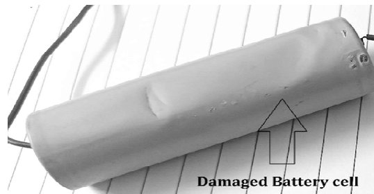
Figure 3: Physically damaged Lithium-ion cell
