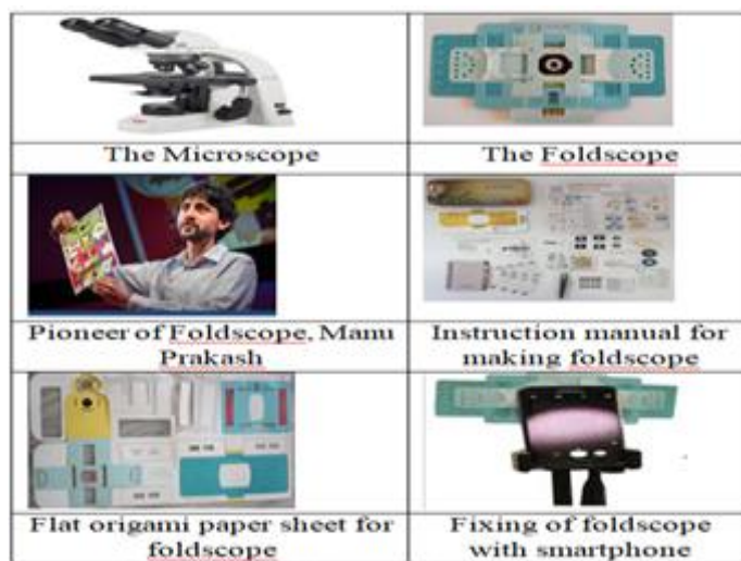
Figure 1: Assembling and handling of foldscope
