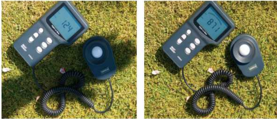
Figure 8: Even in the shade, on a sunny day there is a lot of ambient light around—12,400 lux (1,152 fc) in the measurement shown on the left. Nevertheless, this figure is less than one-seventh of the 87,100 lux (8,092 fc) measured from the direct sunlight on the right. A 7:1 variation in light levels over such a small distance would normally be designed out of the lighting of an interior space, yet this extreme contrast is exactly what natural light is all about. [Source: Lighting for Interior Design Book]
