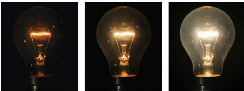
Figure 15: The color of the light produced by the filament is directly related to its temperature. [Source: Lighting for Interior Design]
