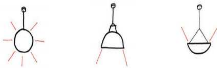
Figure 29: Left: Non- Directional Pendant; Center: Downlight Pendant; Right: Uplight Pendant[Source: Lighting for Interior Design]
