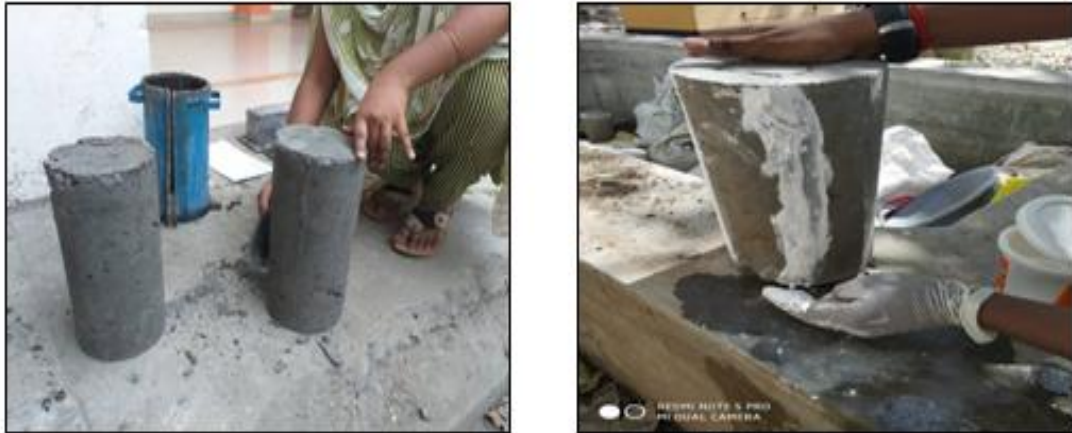
Figure 2: Cylinder Repairing Process
