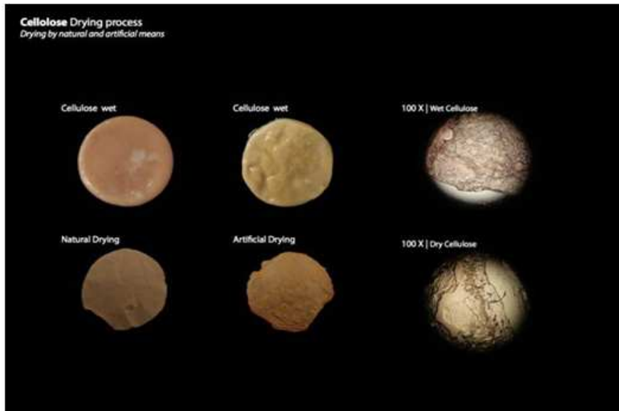
Figure 8: Drying Process of Cellulose (Source: IAAC Blog - Bio-Fabric | Microbial Cellulose)
