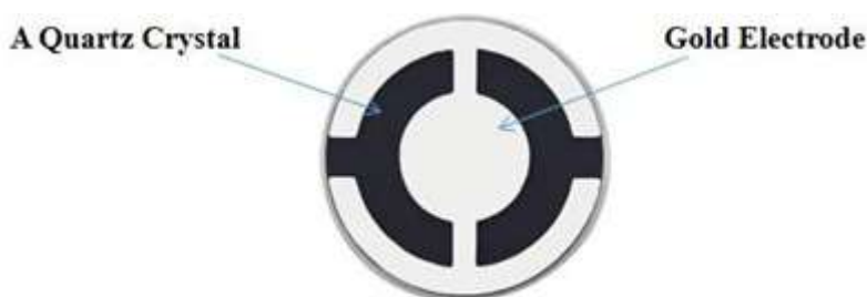
Figure 4: AT-cut quartz crystal with gold electrodes patterned on both sides.
