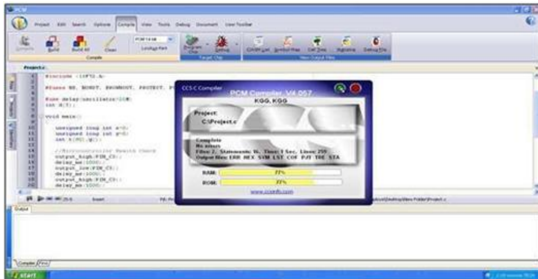
Figure 5: Window Image of Checking Errors and Warnings using the PIC C Compiler
