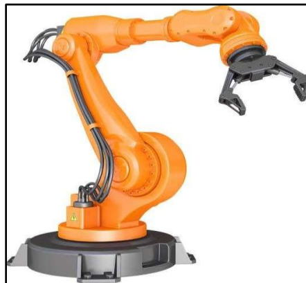
Figure 1: Articulated Robotic Arm
