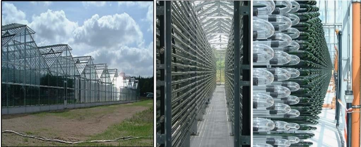
Figure 3: A high-end closed bioreactor system. The world's largest closed photo-bioreactor in Klötze, near Wolfsburg, Germany (Bioprodukte Prof. Steinberg; www.algomed.de ); the 700m 3 are distributed in 500 km of tubes and produce up to 100 t algae biomass per year
