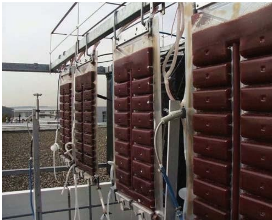
Figure 4: Flat panel airlift from Subitec [38, 102] with usage of the flashing light effect, here for astaxanthin production Triangle Airlift Reactor, or 3D Matrix Algae Growth Engineering Scale Unit, GreenFuel,
