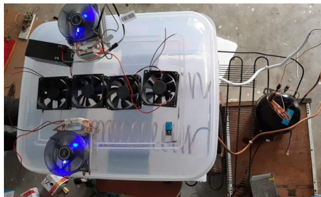
Figure 2: Prototype of thermoelectric dehumidifier based water generator
