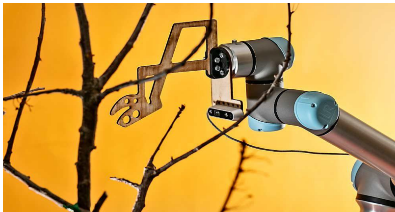
Figure 2: Robotic automated pruning
