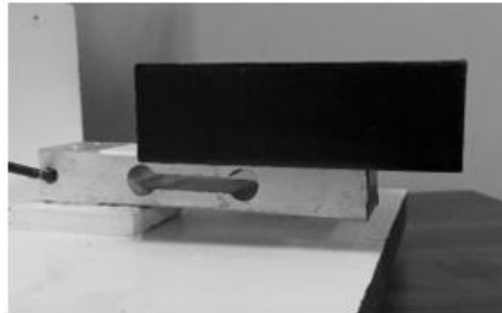
Figure 13: Weighing Module as seen on the prototype
