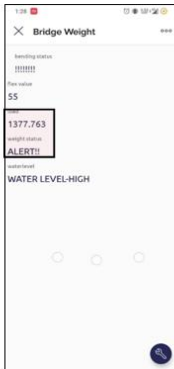
Figure 26: Load on the bridge is more
