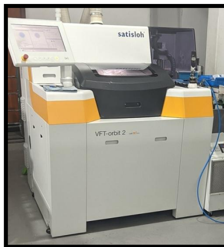
Figure 5: Modern Ophthalmic Lens Making Machine
